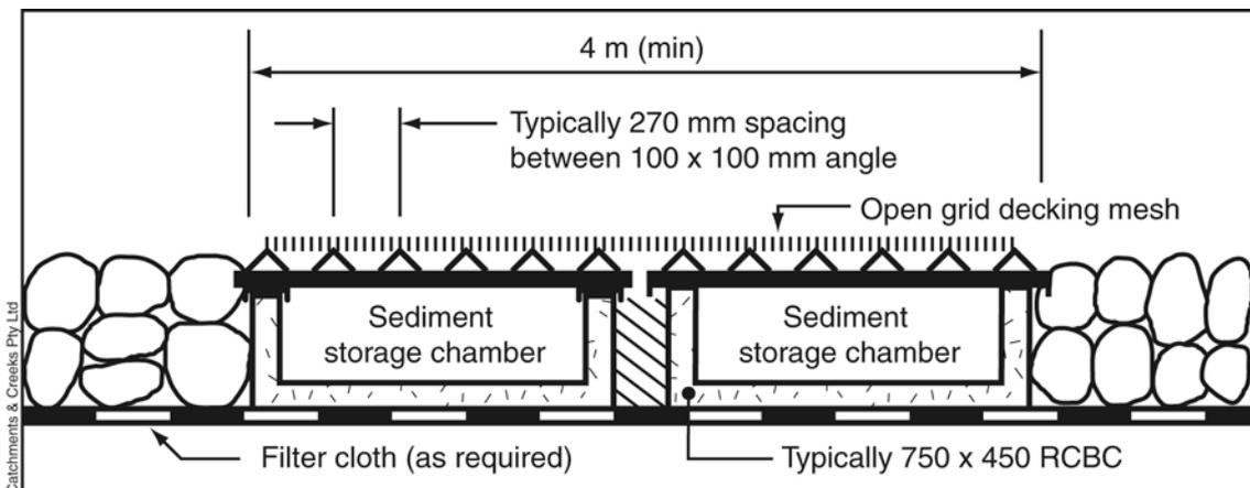
**Figure 5 – Alternative conceptual design using upper mesh layer**
