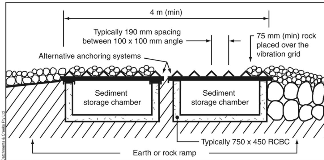
**Figure 4 – Alternative conceptual design using rock upper course**
