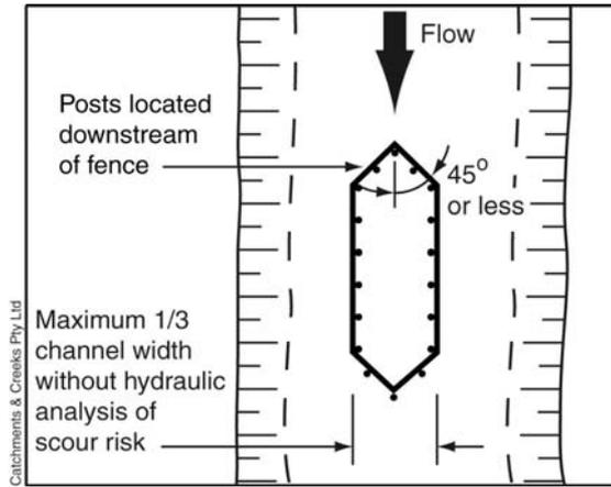
**Figure 2 – Isolation of mid-channel disturbance**
