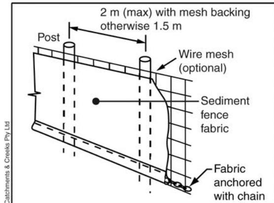
**Figure 4 – Anchorage of riverside isolation barrier using chain ballast**
