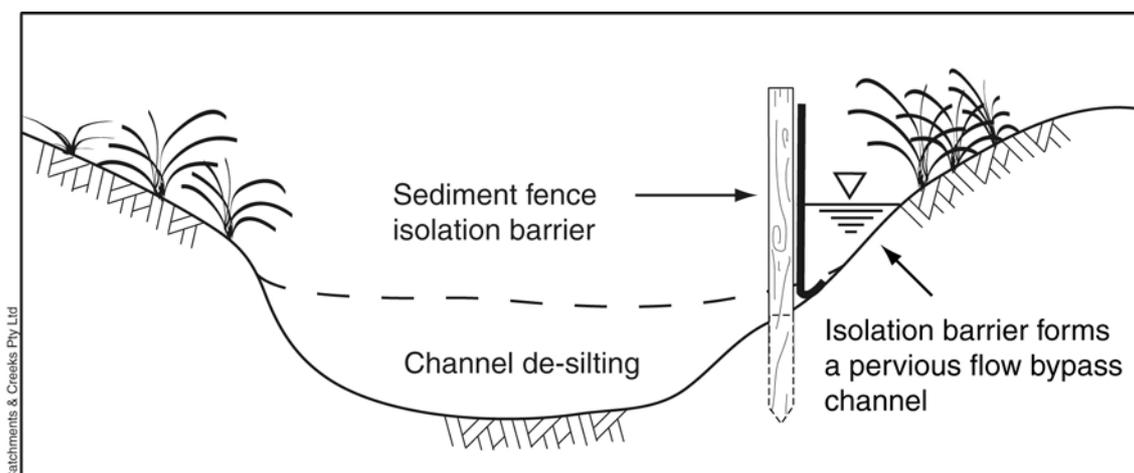
**Figure 7 – Cross-section A-A from Figure 6 (above)**
