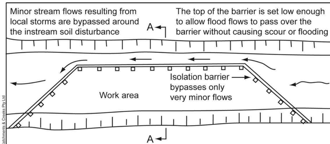
**Figure 6 – Sediment fence isolation barrier used to divert intermittent stream flows**
