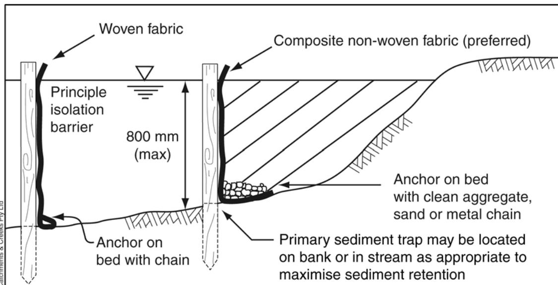
**Figure 5 – Typical installation of sediment fence isolation barrier**
