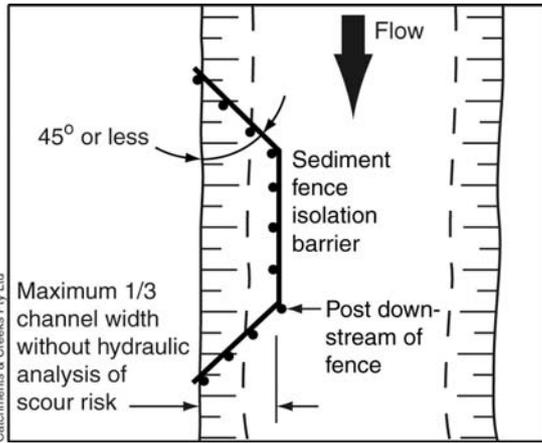
**Figure 1 – Isolation of bank disturbance**
