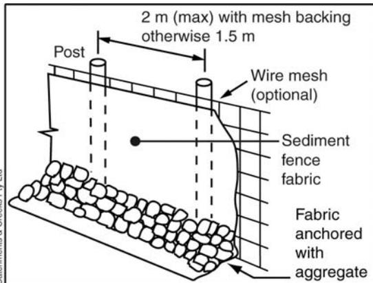
**Figure 3 – Anchorage of landward sediment fence using aggregate**
