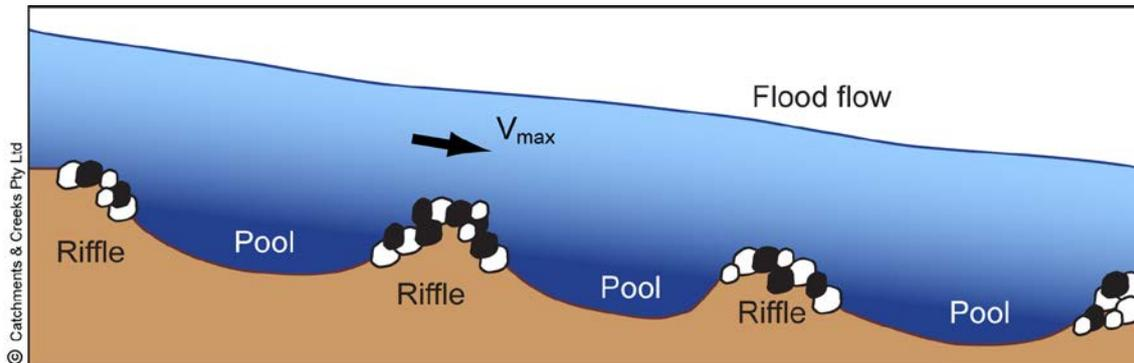
**Figure 2 – Critical high-flow conditions passing over several riffles**
