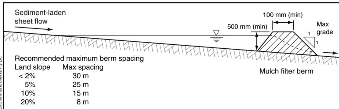
**Figure 1 – Placement of mulch filter berms**
