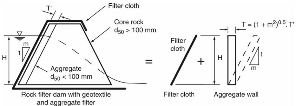
**Figure 9 – Rock filter dam formed from large, free-draining rock with combined geotextile and aggregate filter**
