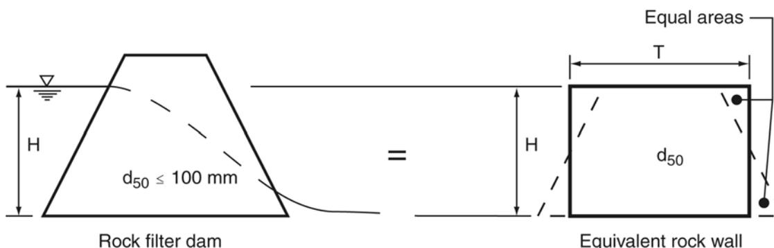
**Figure 5 – Rock filter dams formed only from small filter rock (not recommended)**
