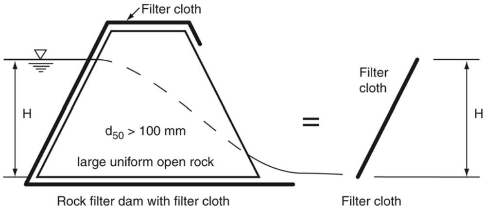
**Figure 7 – Rock filter dam formed from large, free-draining rock with upstream filter cloth**
