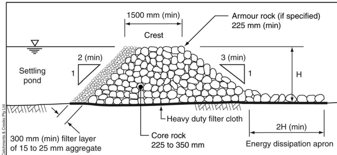
**Figure 1 – Rock filter dam with aggregate filter**
