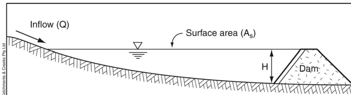
Figure 3 – Minimum design flow condition
