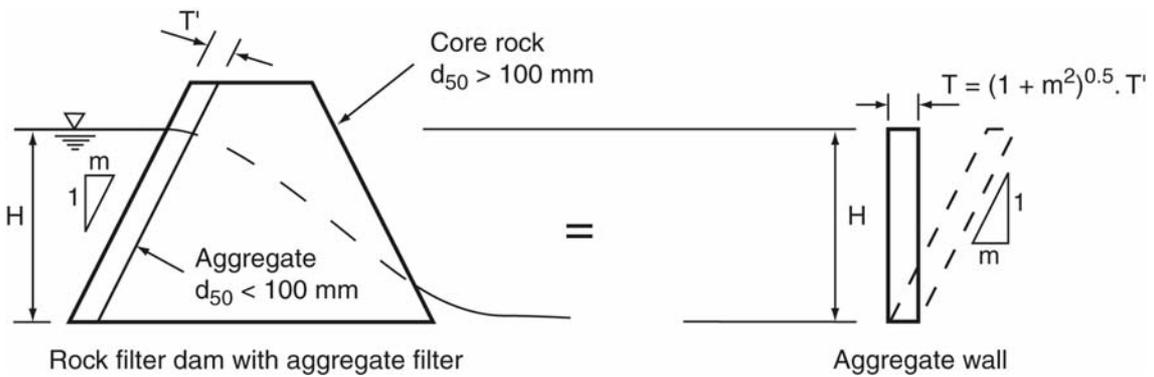
**Figure 8 – Rock filter dam formed from large, free-draining rock with upstream aggregate filter**
