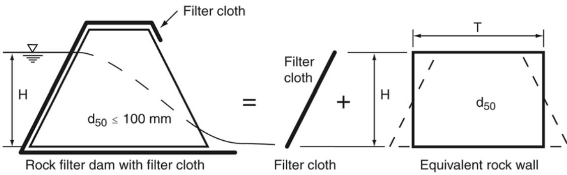
**Figure 6 – Rock filter dam formed from small filter rock with upstream filter cloth**
