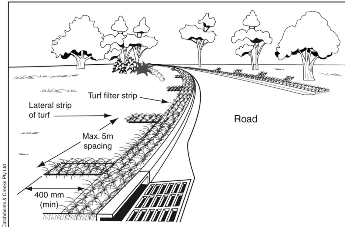
**Figure 1 – Use of lateral strips of turf to control rilling along the up-slope edge of a roadside grass filter strip**
