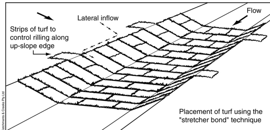
**Figure 2 – Placement of turf in high-velocity drainage channels and chutes**
