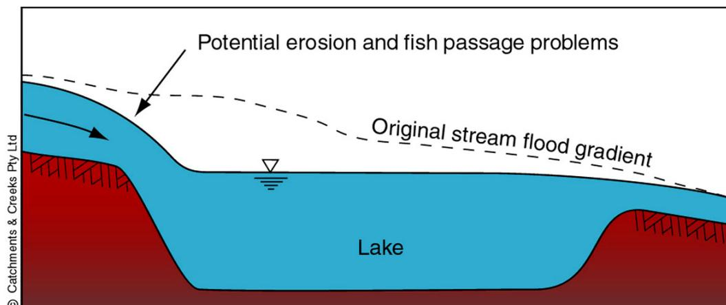
**Figure 1 – Typical water surface gradient of an on-stream constructed lake**
