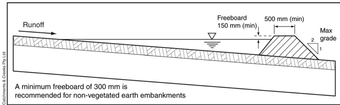
**Figure 2 – Flow diversion bank formed from earth**
