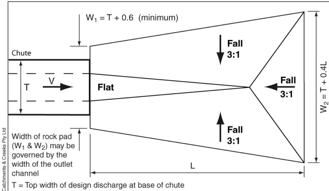
Figure 2 – Typical arrangement of a recessed outlet structure (plan view)
