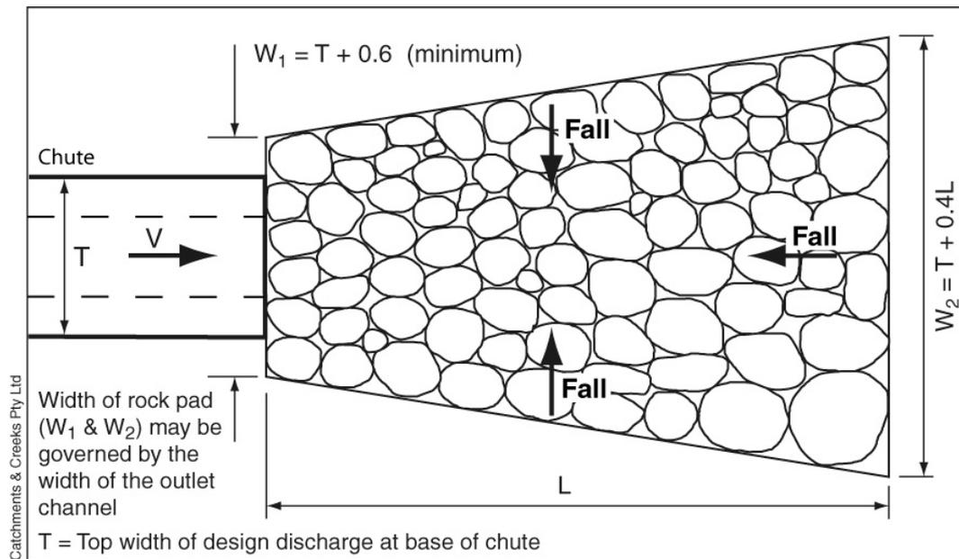
**Figure 1 – Typical layout of a recessed rock pad for a chute (plan view)**
