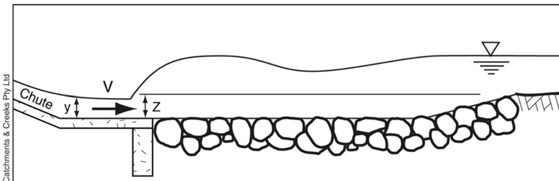
Figure 3 – Typical profile of a recessed outlet structure (side view)
