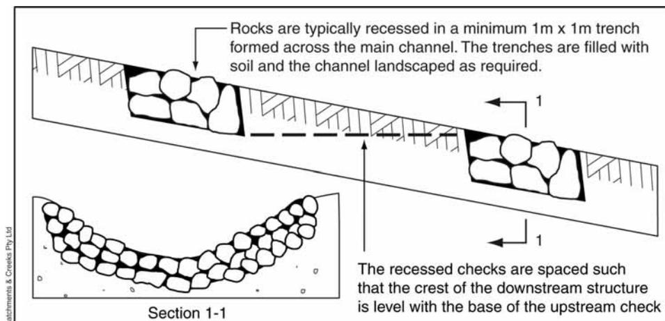
**Figure 4 – Fully recessed rock check dams**
