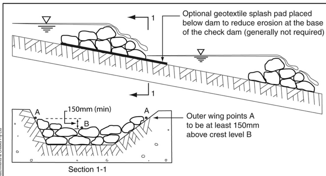
Figure 1 – Profile of temporary check dams
