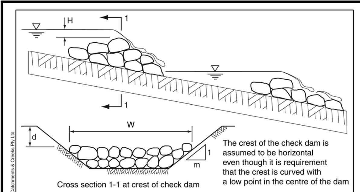
**Figure 2 – Assumed check dam profile for Equations 1 and 2**
