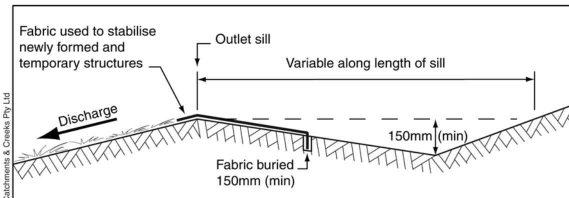
Figure 4 – Cross-sectional profile of end sill
