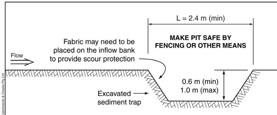
**Figure 1 – Minimal dimensional requirements of excavated sediment trap located within a minor drainage path**
