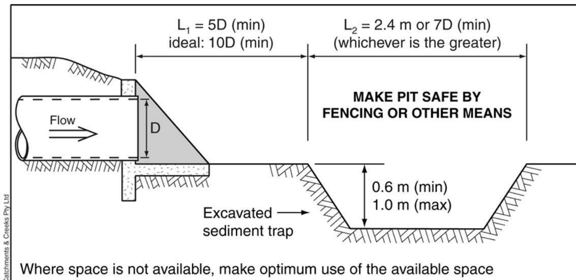
**Figure 2 – Ideal minimal dimensional requirements of excavated sediment trap located downstream of a stormwater outlet**
